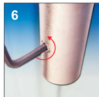
6 Loosen the set screw with 2,5 mm Allen key.
