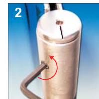
2 Loosen the set screw with 2,5 mm Allen key.
