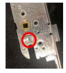
Push down on the screw driver as you pull out on the strike until the strike is released
