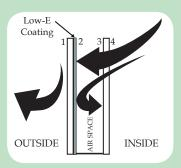
In cold weather conditions, the coating on the #2 surface reduces room heat (or infrared energy) from transferring across the airspace toward the outside. By adding a second Low-E coating to the #4 surface the thermal insulation is improved.
