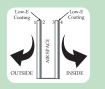
A Low-E coating on the #4 surface reflects room heat, back inside in cold weather conditions. This reduces the radiant heat loss and improves the overall insulation of the IGU.
